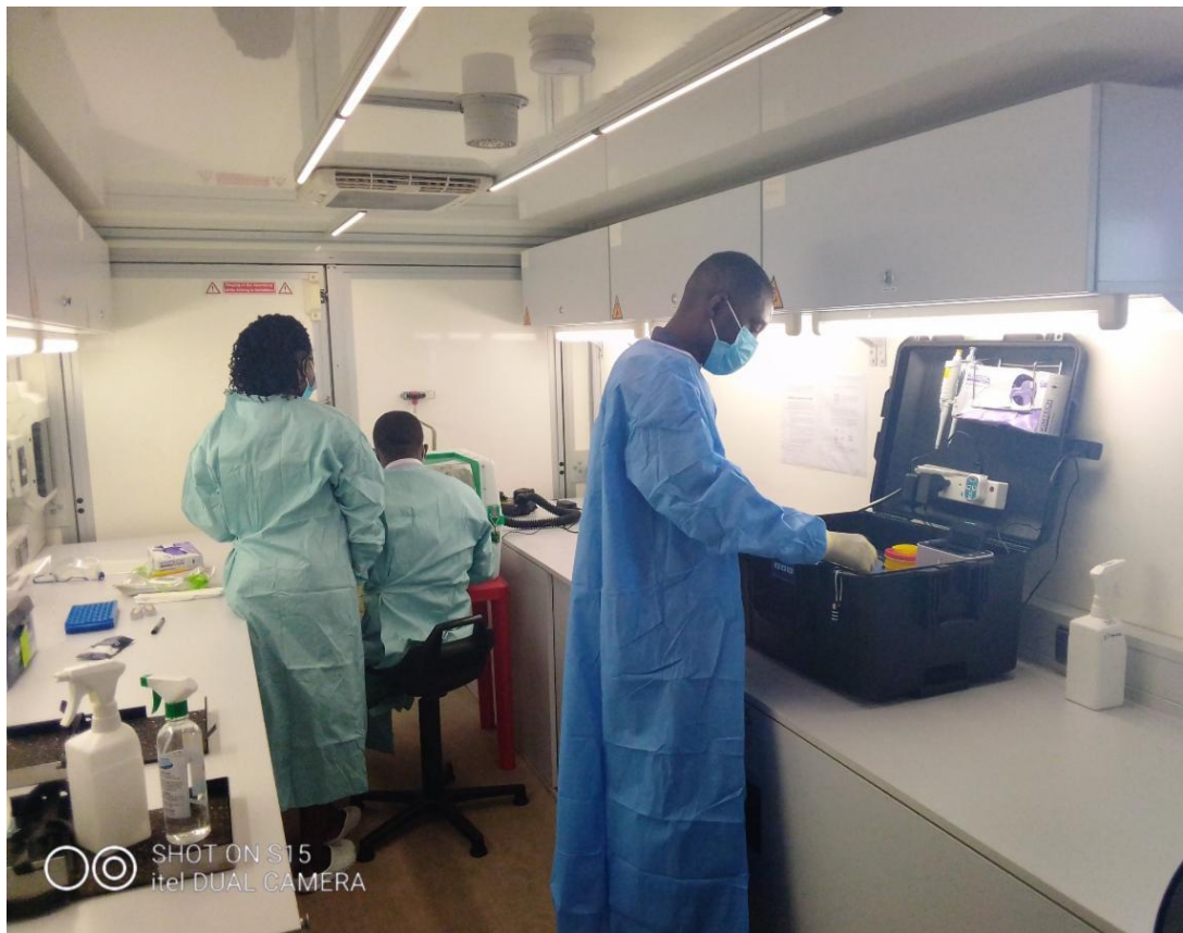
The team working inside the mobile van laboratory. The lab is fitted with a glovebox for inactivation and RNA extraction, a suitcase lab with a real-time PCR machine for amplification.
