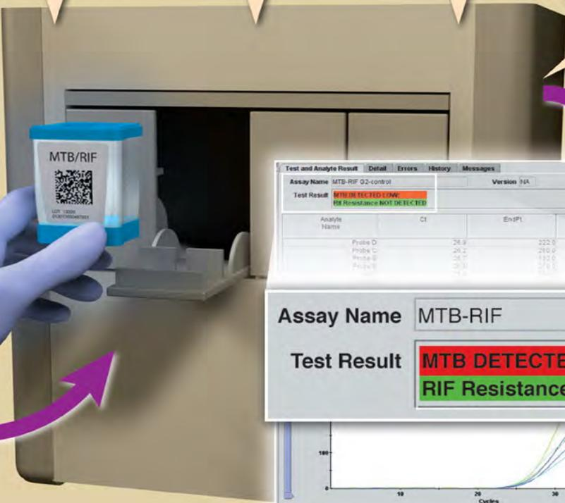
3 Cartridge inserted into MTB-RIF test platform (end of hands-on work)
